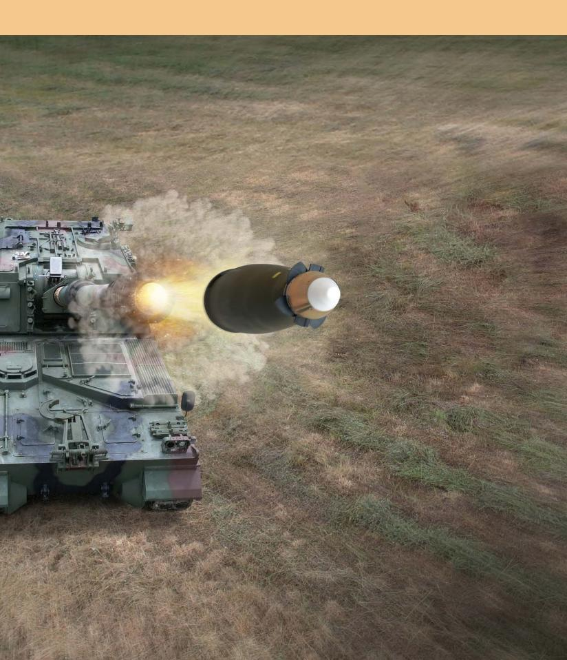
**155 mm Howitzer Ammunition Range Correction Kit [MDK]** is a guidance kit that can be used instead of the standard fuzes of unguided artillery ammunition, reducing the range probable error to 50 m.
