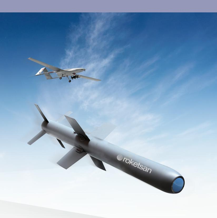
MAM-C lightweight Smart Micro Munition has been developed for unmanned aerial vehicles [UAV] and light attack aircraft, and for air-to-ground missions where weight is a critical factor.
