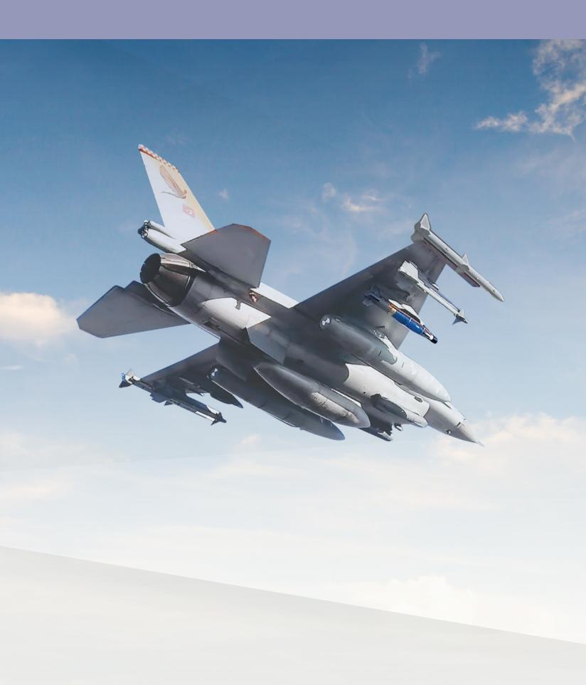
**LAÇİN guidance kit** can be used against fixed and mobile targets with its imaging infrared seeker and data link. LAÇİN, in which the pilot is kept in the loop via L-POD, is compatible with MK-82 generalpurpose bombs. The guidance kit transforms General-Purpose Bombs into smart weapon systems through the integration of an Inertial Measurement Unit [IMU], a Global Positioning System [GPS] and an Infrared Seeker.
