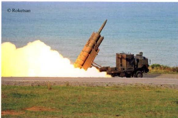
T – 300 ÇNRA is a 300 mm, multi barrel Rocket Launcher system fitted with the latest sub – systems, which are capable of effectively firing at critical targets, 100 km in depth.
